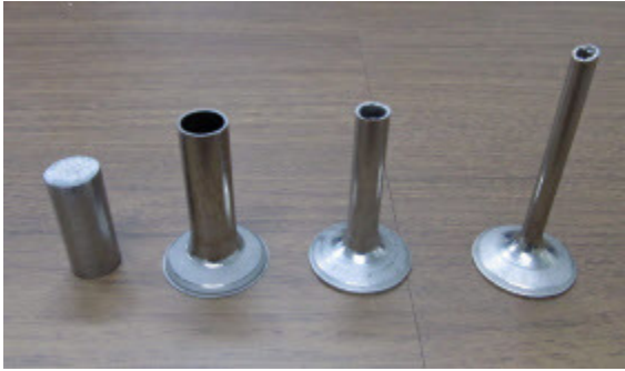
Working process to form the (rightmost) engine valve with a hollow umbrella portion Figure 5
