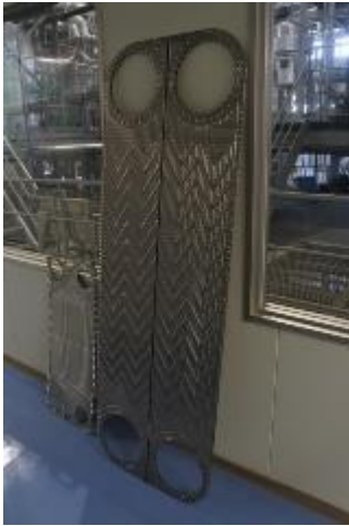
Figure 6 • Plate components for heat exchange displayed in Imari Satellite
